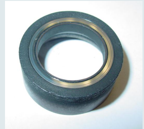
Mating Ring with Coke from High Heat Generation
